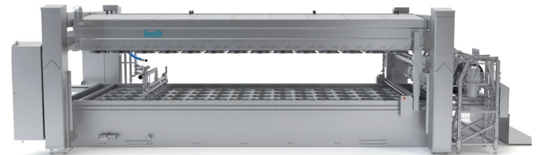
The patented Kalt cassette press is designed for single and multi-batch operation. The curd is automatically flushed into the round or square moulds, gently pressed, and discharged from the moulds onto a conveyor belt for further treatment.
